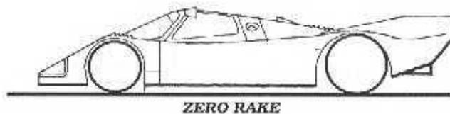
Rake is the tilt of the chassis from level in side view.
